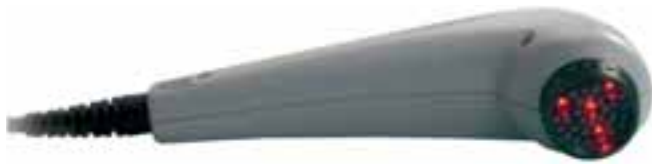
FIG 12-16 A cluster light applicator that includes LEDs that emit low-power red light and SLDs that emit higher power infrared light. Courtesy Dynatronics, Salt Lake City, UT.
