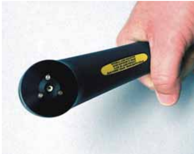
FIG 12-17 A laser diode applicator. This applicator includes one infrared laser diode and three blue LEDs that serve as indicators to show when the applicator is on. Courtesy Mettler Electronics, Anaheim, CA.
